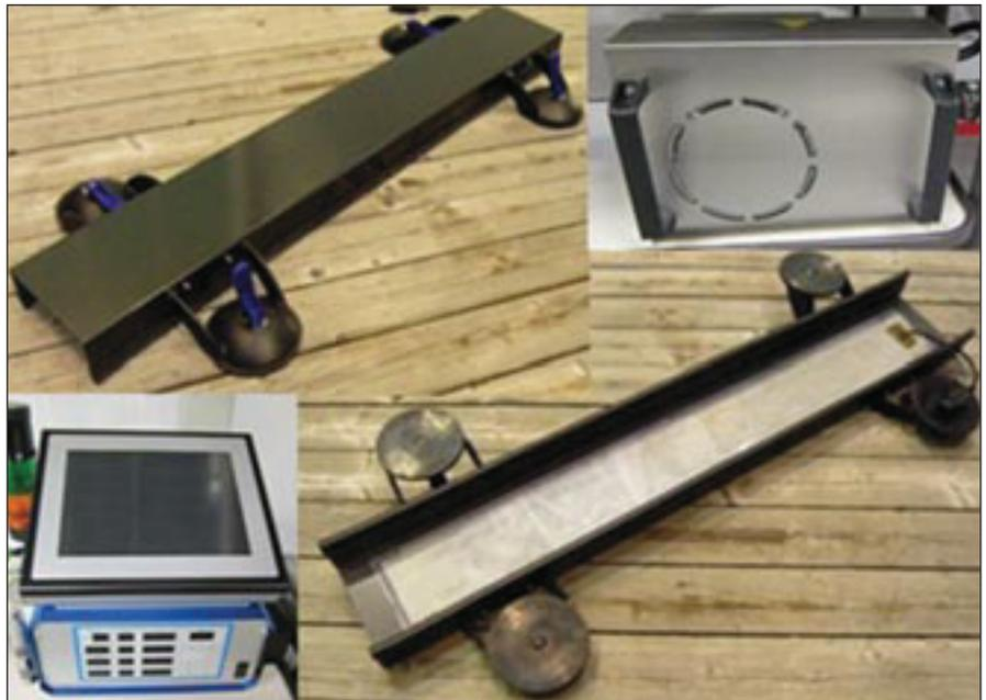
The prototype heated air tube system, bottom view (top left), inside view (bottom right), ventilating fan (top right), and control unit (bottom left).
