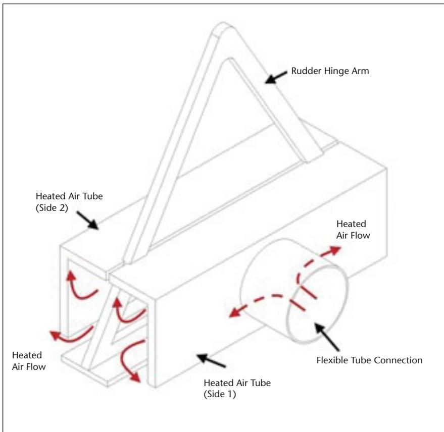
Schematic representation of the heated air system for accelerated curing of shim.
