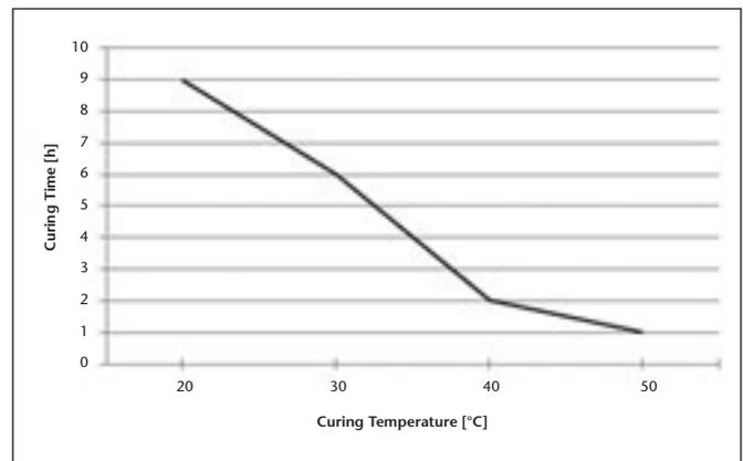
Curing time of the used shim material dependent on the curing temperature.
