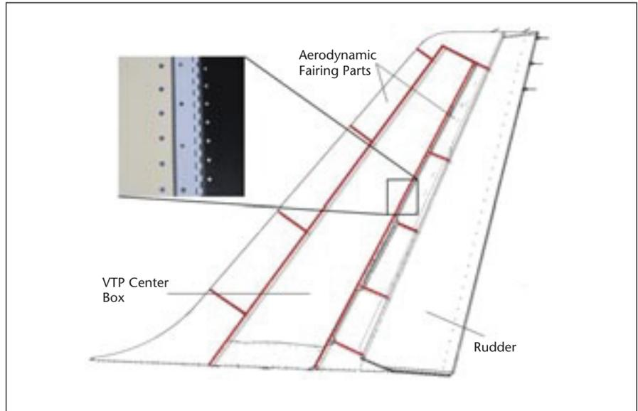
Vertical tail plane (VTP) of a single-aisle passenger aircraft showing gaps on the outer surface (in red) that have to be filled by aerodynamic sealing.
